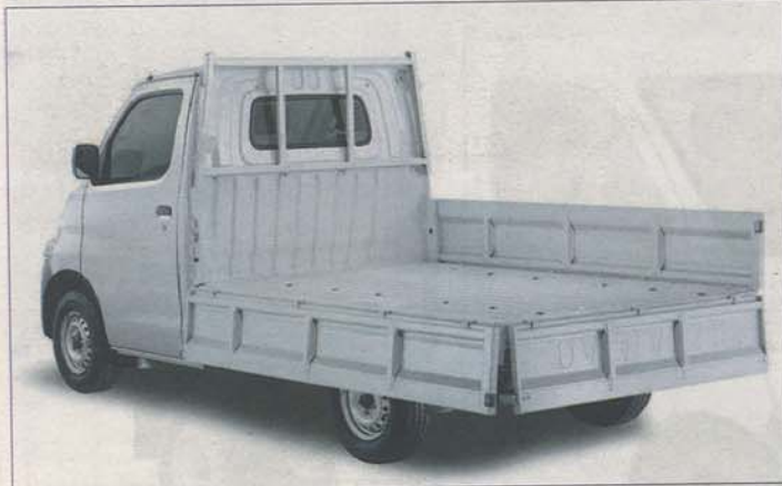
For ease of use, the loadbay sports no less than three dropsides. Photos - Daihatsu
